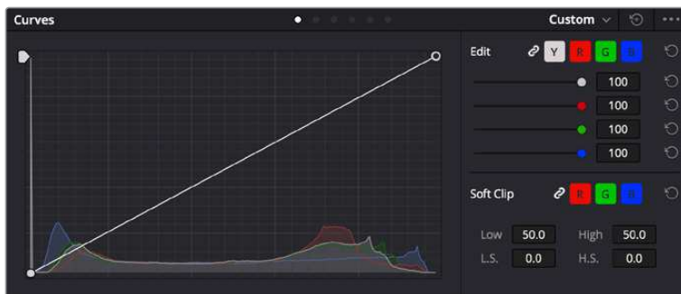
The curves palette is another tool you can use to make primary color corrections, or enhance specific areas of your clip when using a power window
